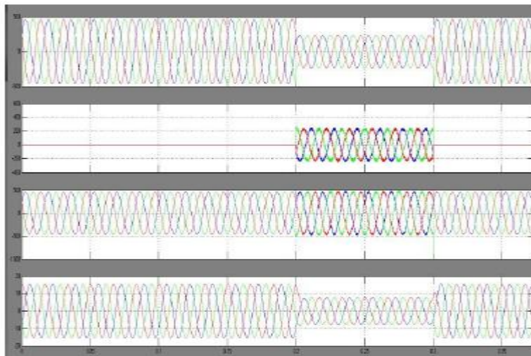
Figure 7 Simulation waveforms of source voltage, DVR voltage, load voltage, source current using PI controller
